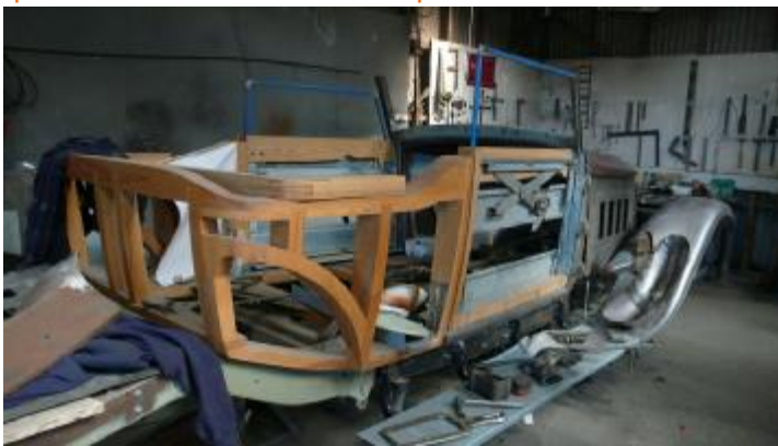
Bottom 5 photos: Michael & Mary Taylor's 1930 Packard Waterhouse bodied replica ((3 rd of the 3 sisters!). Work continues, motor half way, overdrive fitted. Body now being skinned. Doors now lining up, and chassis has been extensively repaired with much of the front replaced.
