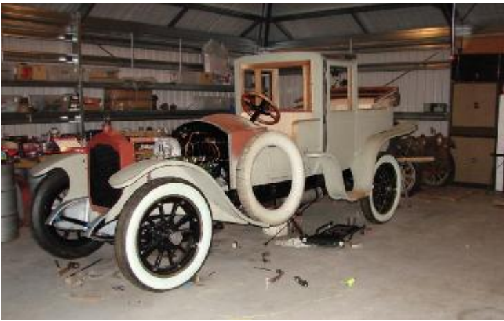
Bottom 5 photos: Michael & Mary Taylor's 1930 Packard Waterhouse bodied replica ((3 rd of the 3 sisters!). Work continues, motor half way, overdrive fitted. Body now being skinned. Doors now lining up, and chassis has been extensively repaired with much of the front replaced.
