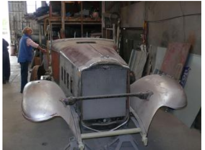
Bottom 5 photos: Michael & Mary Taylor's 1930 Packard Waterhouse bodied replica ((3 rd of the 3 sisters!). Work continues, motor half way, overdrive fitted. Body now being skinned. Doors now lining up, and chassis has been extensively repaired with much of the front replaced.
