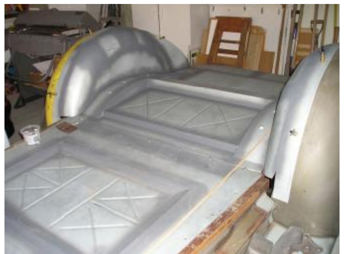
All panels from the windscreen back, and the floor, have been wheeled up by Dallas on the wheeling machine he made. What a wonderful job Dallas has done so far - we cannot wait to see the finished car - Ed
