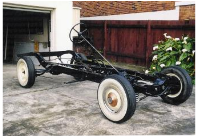
Completed chassis waiting for engine and body
