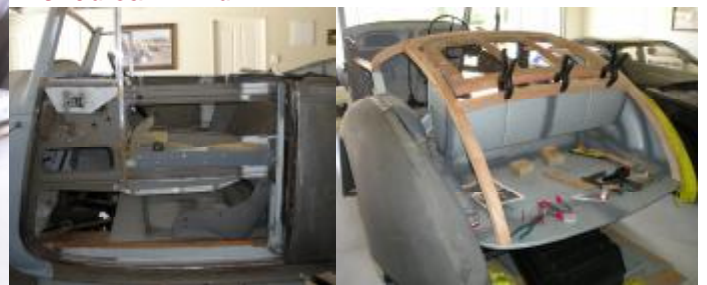
All panels from the windscreen back, and the floor, have been wheeled up by Dallas on the wheeling machine he made. What a wonderful job Dallas has done so far - we cannot wait to see the finished car - Ed
