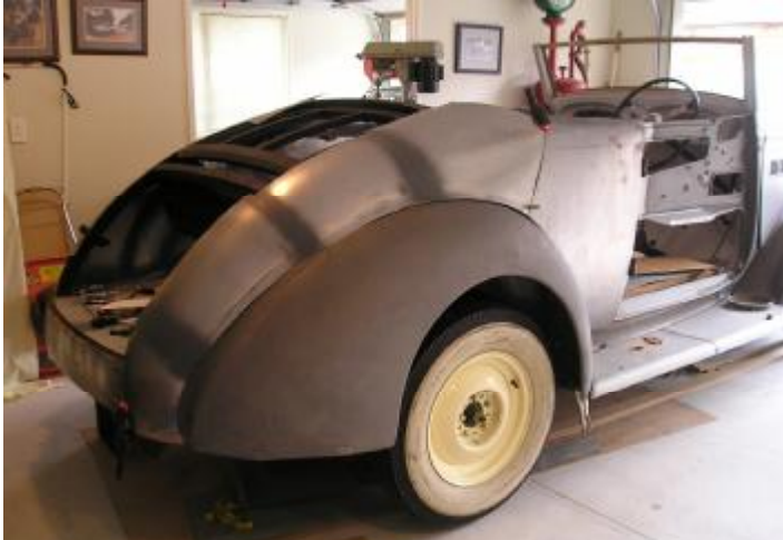
All panels from the windscreen back, and the floor, have been wheeled up by Dallas on the wheeling machine he made. What a wonderful job Dallas has done so far - we cannot wait to see the finished car - Ed
